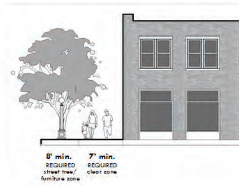
Figure 3-5: TOD Core Transit Corridor sidewalk requirements. Street trees are required along TOD Core Transit Corridors with an average spacing not greater than 30 feet on center.
