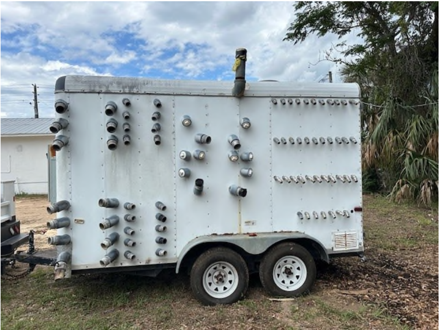
Imperial's Reliable 2006 (T-4) 12'-3"L. x 7'-1"W. Remedial System ready to be mobilized Off-site, fitted with (40) 1" Sparge Pts, (32) Total, (14) 3", and (18) 2" Extraction Pts with (6) x 3" Vapor Carbon Bypass connections, and 3-phase 208-230V, 200A Shut-off.
