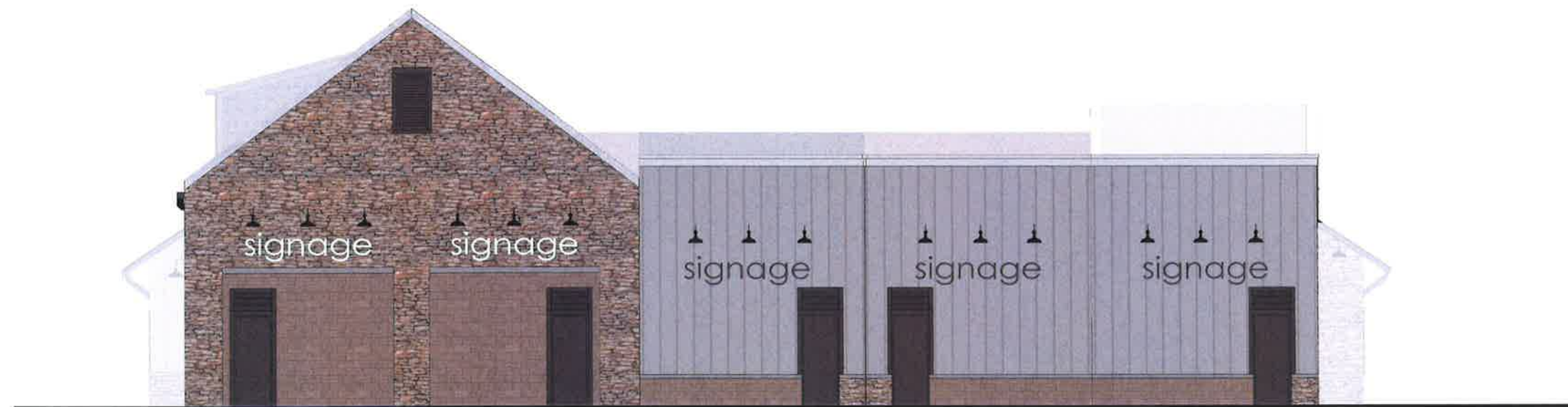
Rear Elavation Building B SCALE: 3/16" = 1'-0"
