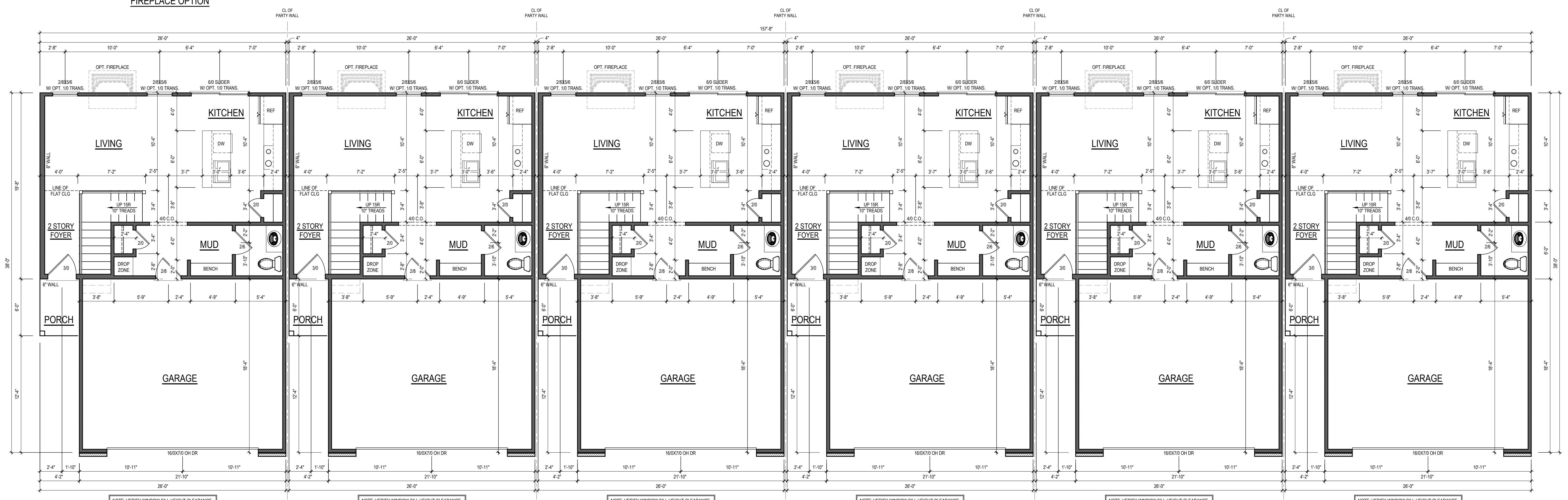
FIRST FLOOR PLAN - ELEV. A 3/16" = 1'-0" CEILING HGT. = 9'-0" FIRST FLOOR PLAN - ELEV. C 3/16" = 1'-0" CEILING HGT. = 9'-0" FIRST FLOOR PLAN - ELEV. A 3/16" = 1'-0" CEILING HGT. = 9'-0" FIRST FLOOR PLAN - ELEV. C 3/16" = 1'-0" CEILING HGT. = 9'-0" FIRST FLOOR PLAN - ELEV. A 3/16" = 1'-0" CEILING HGT. = 9'-0" FIRST FLOOR PLAN - ELEV. C 3/16" = 1'-0" CEILING HGT. = 9'-0"
