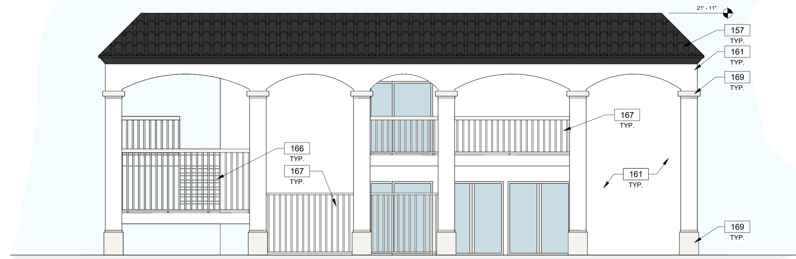
3 BUILDING A SOUTH ELEVATION 3/16" = 1'-0"
