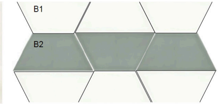
ACCENT TILE - B1 Florida Tile, Emotive, Astonished White (Grout - Laticrete 89 Smoke Grey)
