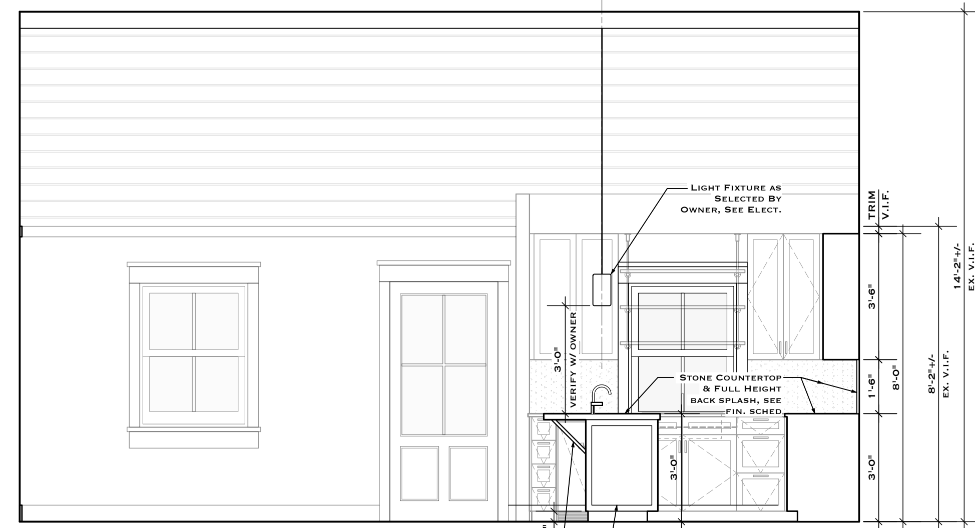
1 INTERIOR ELEVATION - LIVING & KITCHEN AS.1 SCALE: 3/8" = 1'-0"
