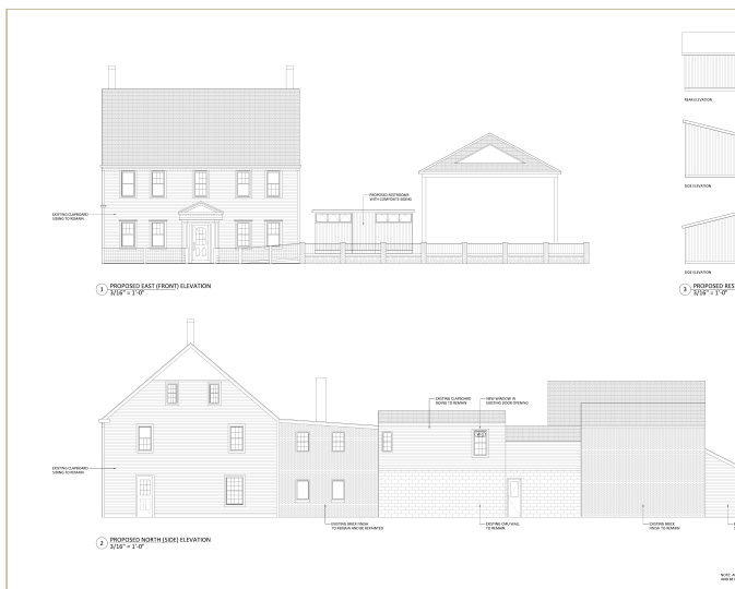
PROPOSED EAST ELEVATION (BANK STREET) & OUTDOOR PAVILION
