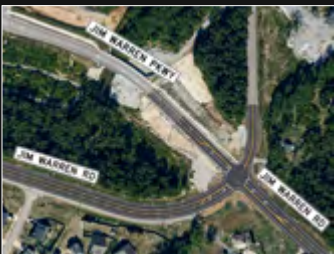
JIM WARREN RD. Realignment from Current Alignment
