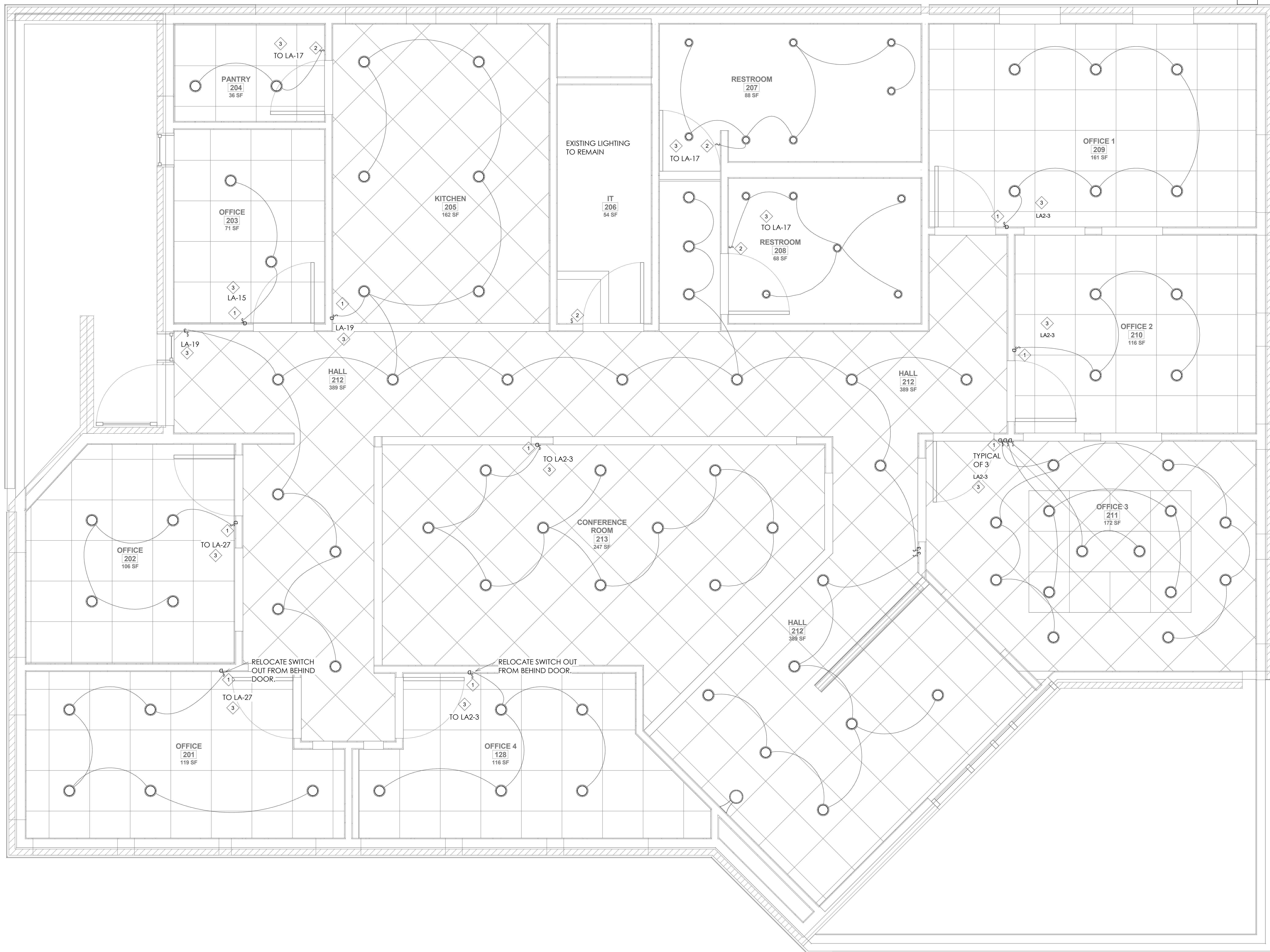
1 LEVEL 2 - ELECTRICAL LIGHTING 1/2" = 1'-0"
