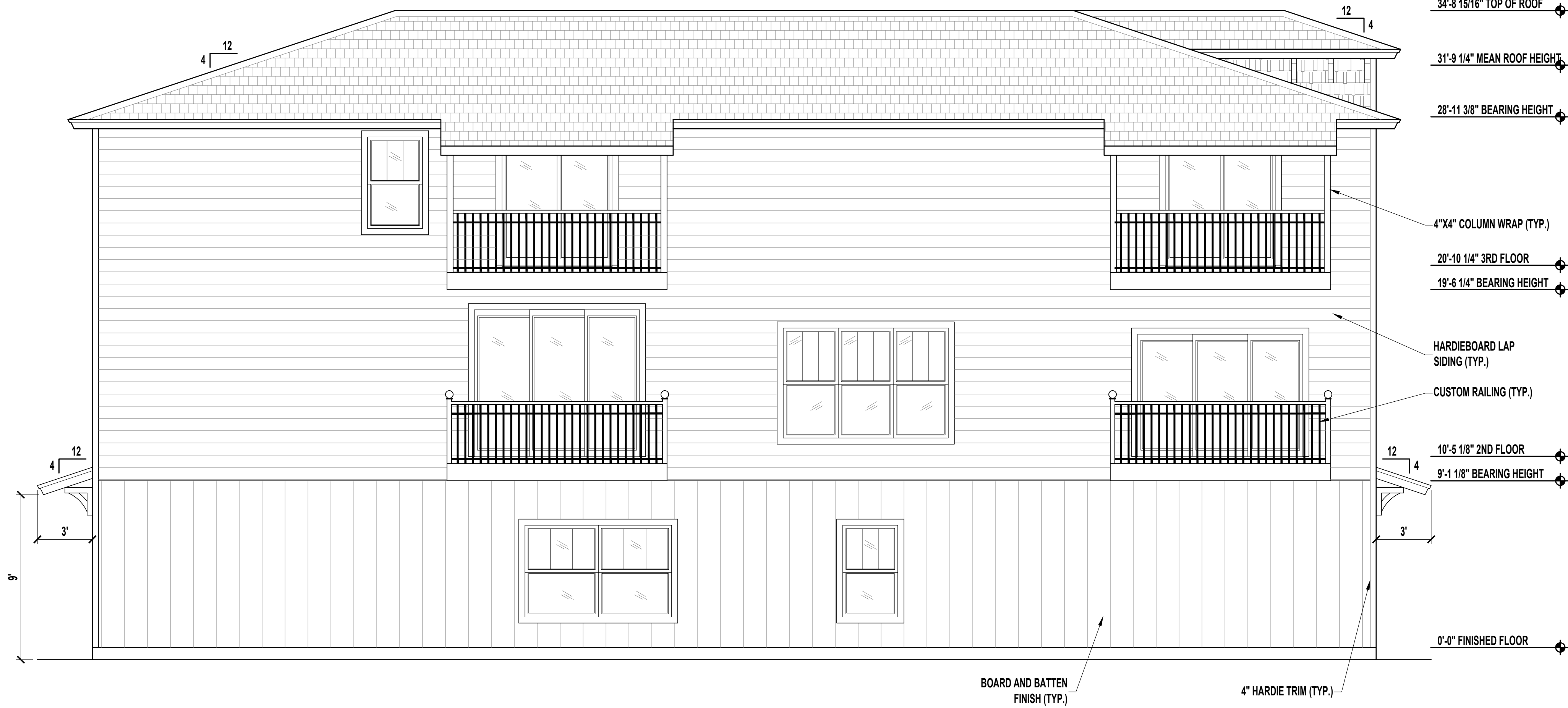
LEFT SIDE ELEVATION SCALE: 1/4" = 1'-0"
