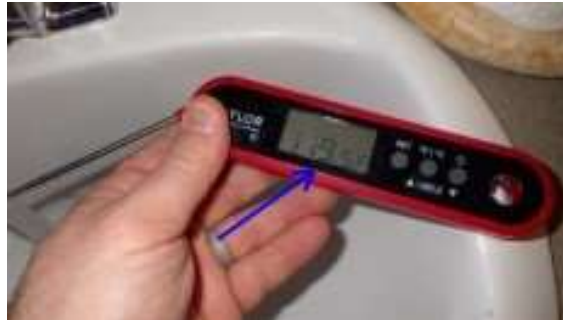
119 degrees F at sink.
