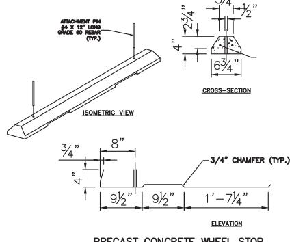
PRECAST CONCRETE WHEEL STOP (TYPICAL)
