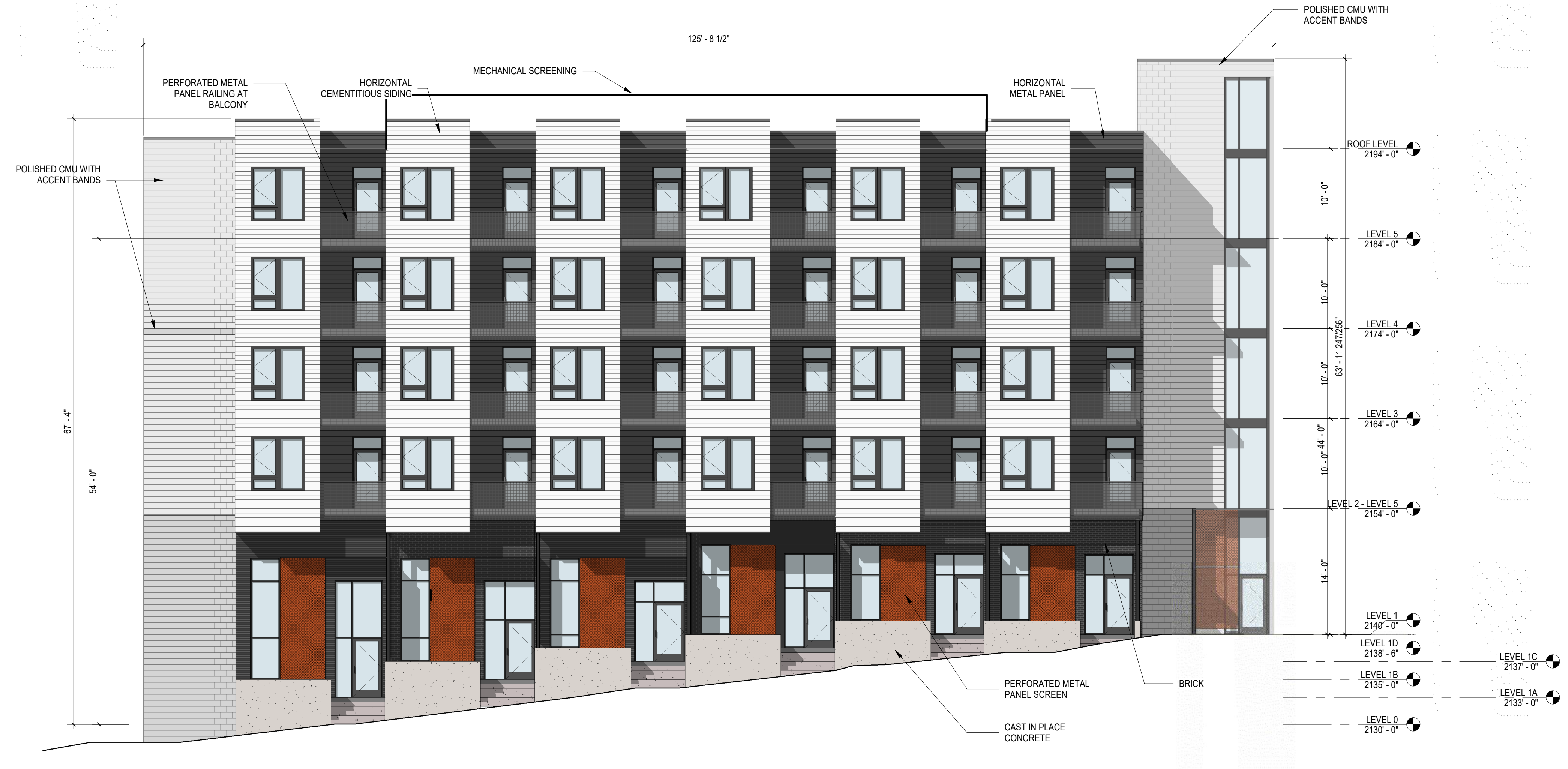
3 SE ELEVATION (COLLIER STREET) A100 1/8" = 1'-0"
