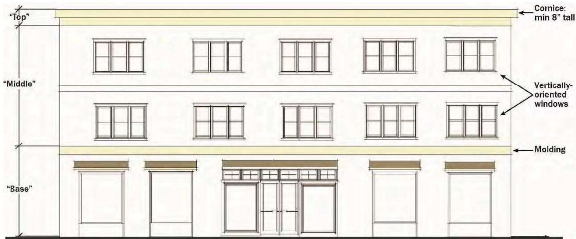
FIGURE 524-2. BUILDING FAÇADE ARTICULATION
