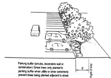
STREETSCAPE PLATE TYPE S-10 MODIFIED (no sidewalks required)
