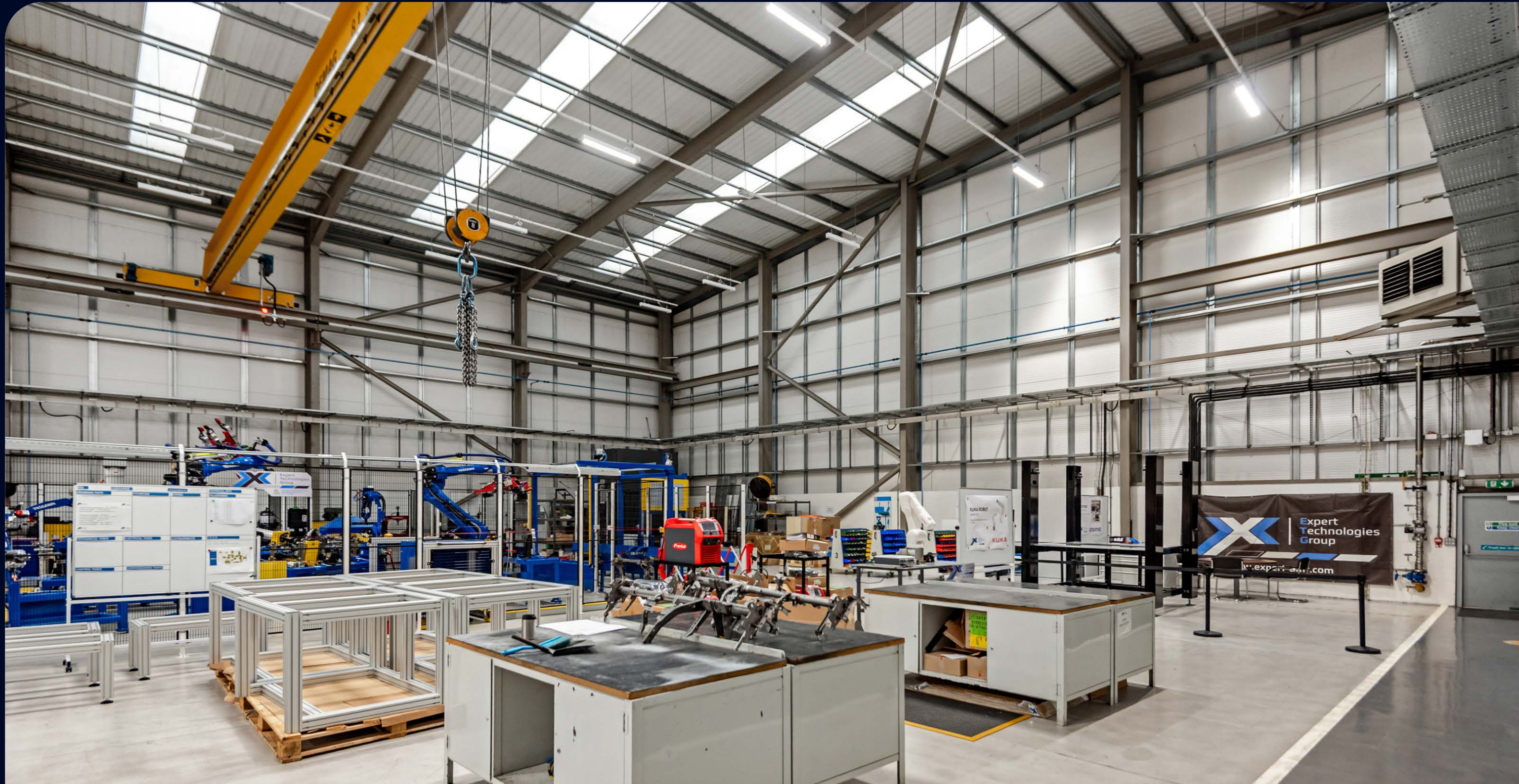
Warehouse with two 8 tonne gantry cranes within the warehouse which are 7m to underside of beam
