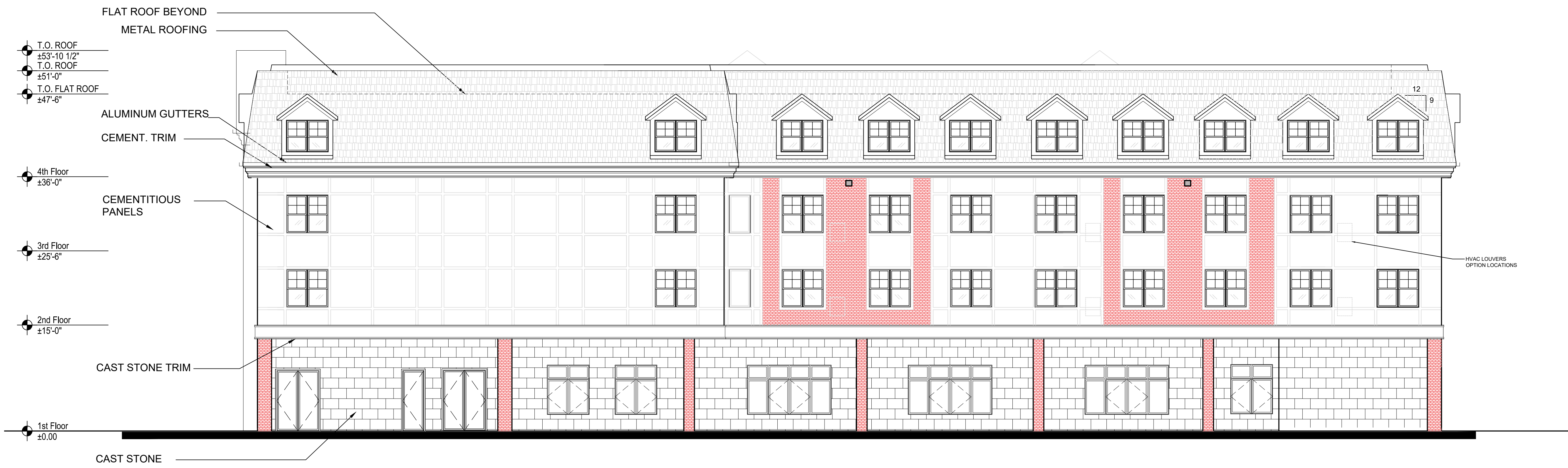
SIDE ELEVATION - SOUTH ELEVATION (PARKING LOT) SCALE: 1/8"=1'-0"
