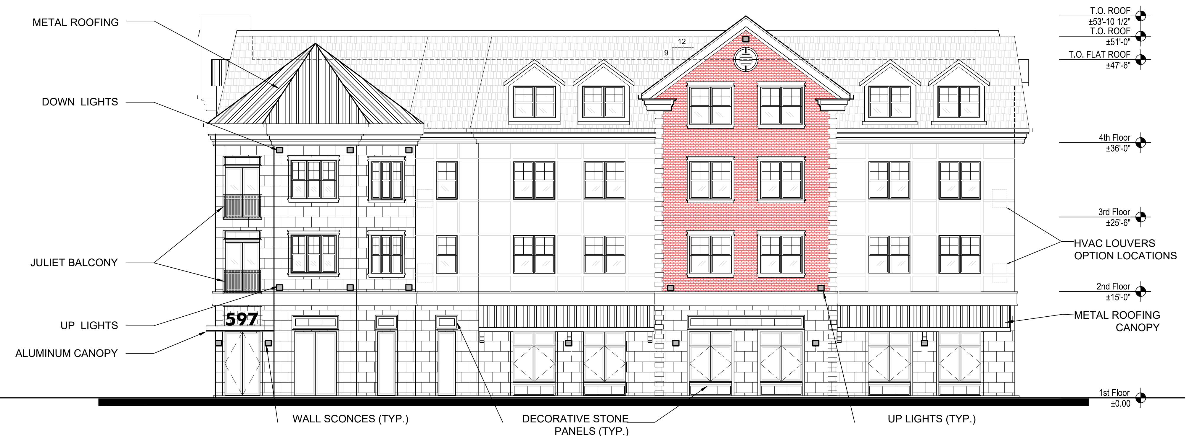
FRONT ELEVATION - WEST (BALTUSROL WAY) SCALE: 1/8"=1'-0"
