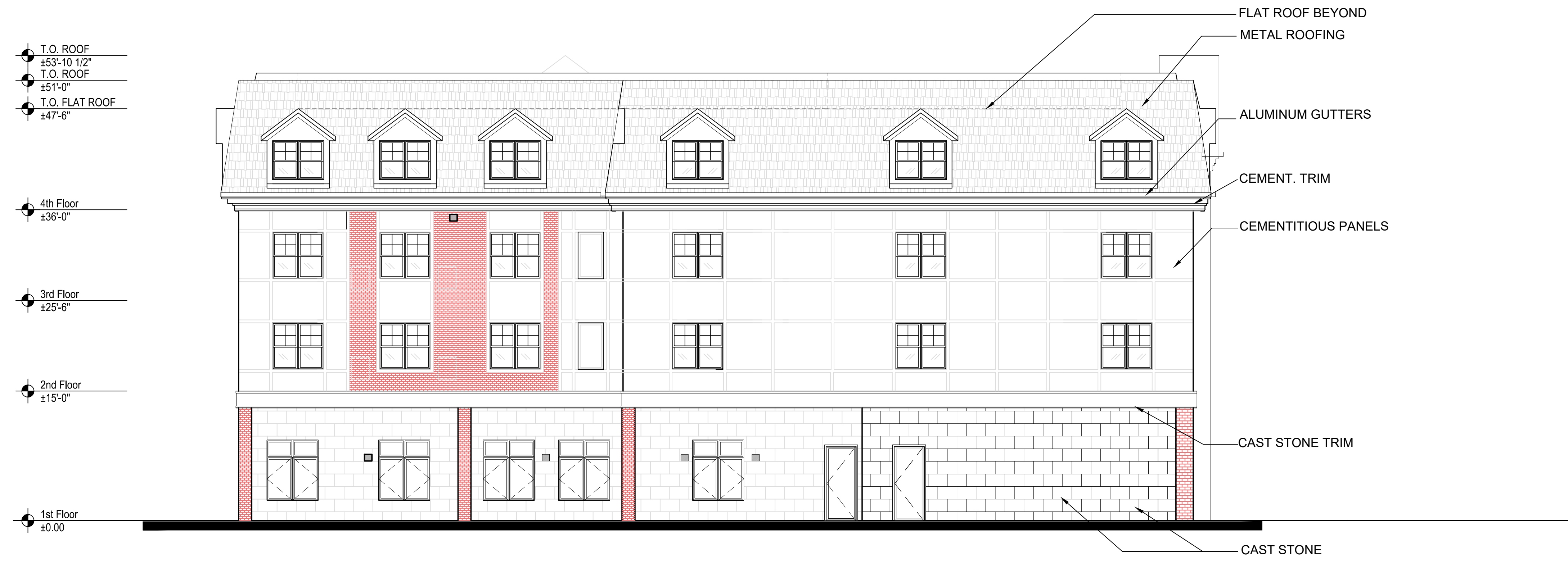
LEFT SIDE ELEVATION - EAST ELEVATION SCALE: 1/8"=1'-0"
