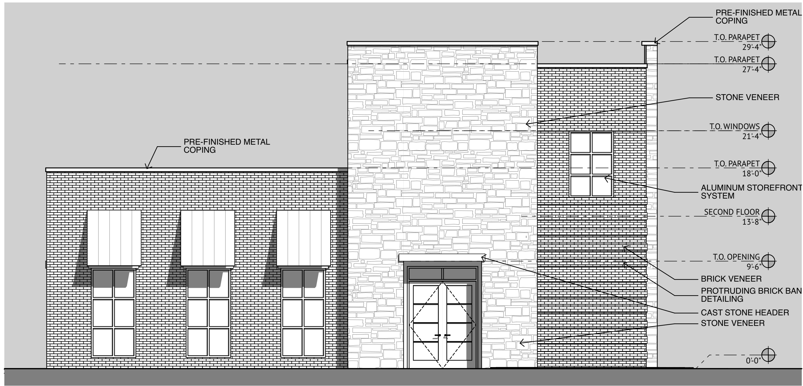
1 BUILDING 3 NORTH ELEVATION SCALE: 3/16" = 1'-0"
