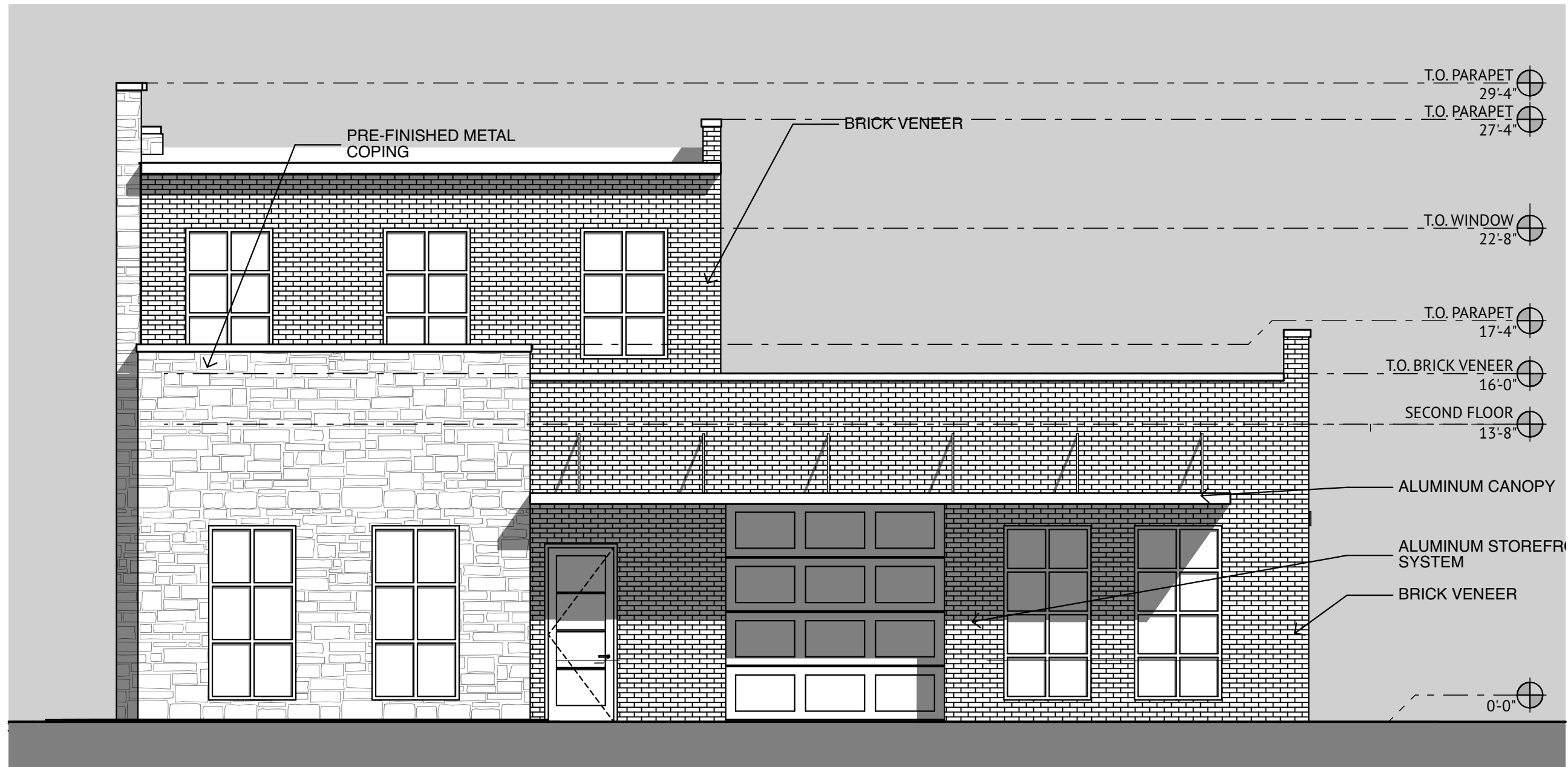
3 BUILDING 3 SOUTH ELEVATION SCALE: 3/16" = 1'-0"
