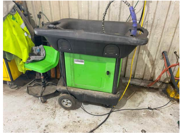
Photo 8 View of an on-site parts washer (Tract 1)
