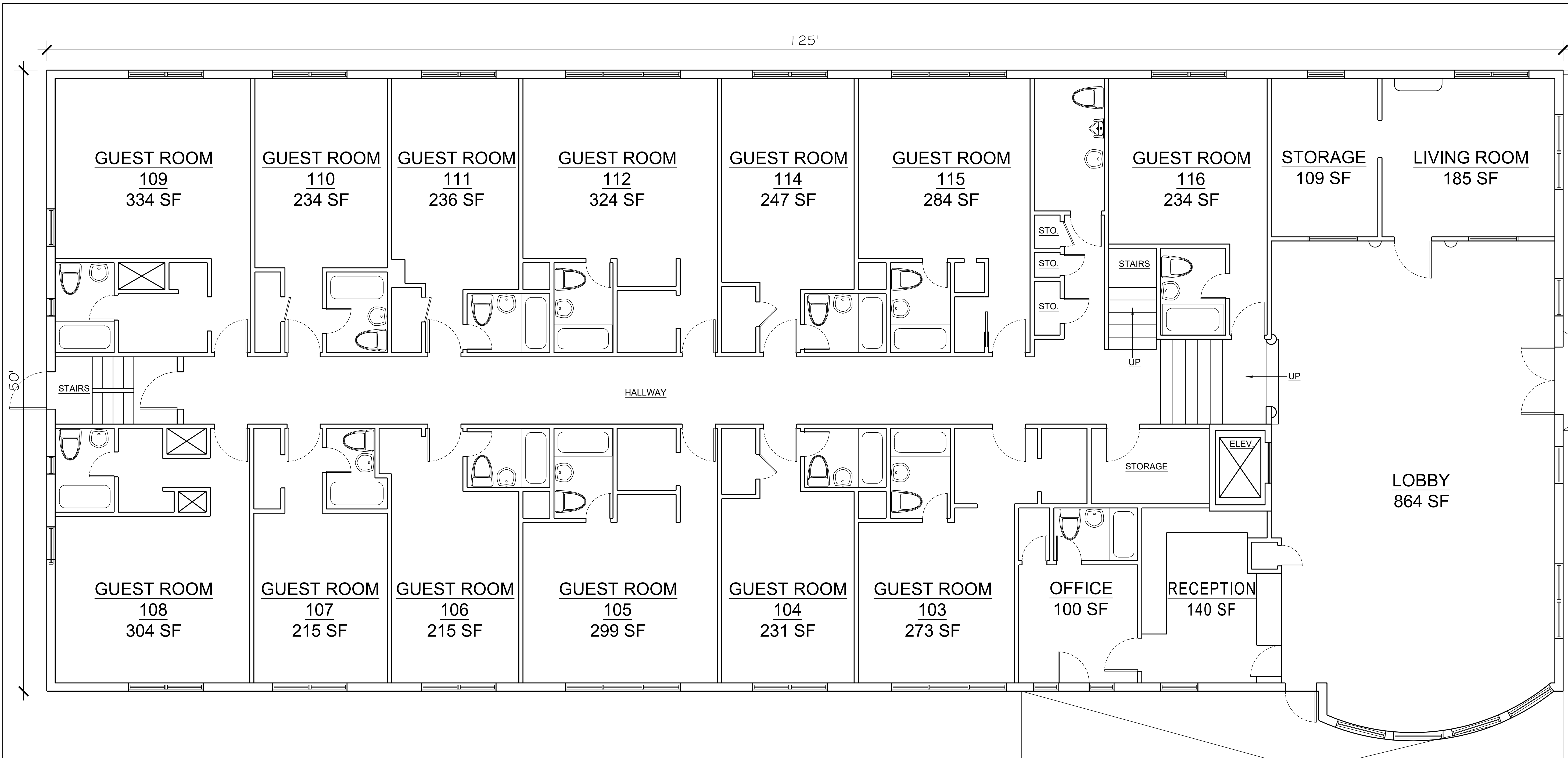
1 FLOOR PLAN - GROUND FLOOR PLAN 1/4" = 1'-0" (13 ROOMS TOTAL)
