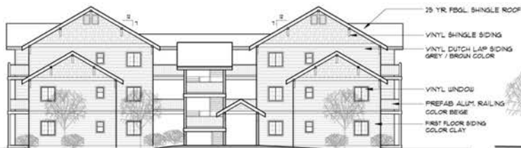
SIDE BUILDING ELEVATION SCALE: 3/32" = 1'-0"
