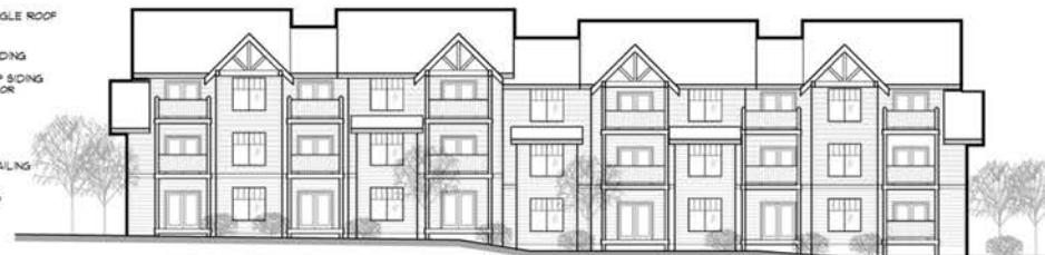
FRONT BUILDING ELEVATION SCALE: 3/32" = 1'-0"
