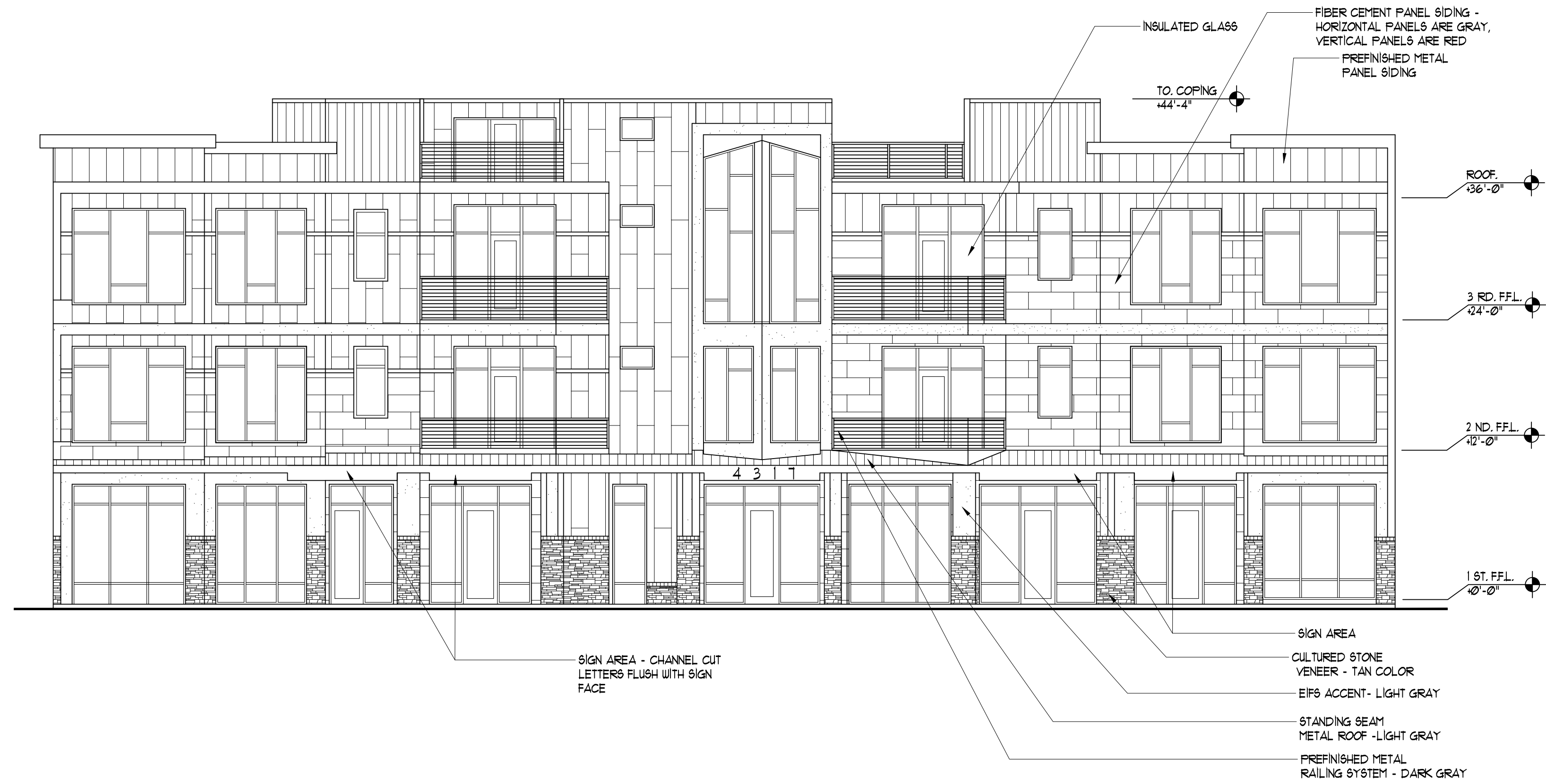
SOUTH ELEVATION (FRONT) 1/8" = 1'-0"
