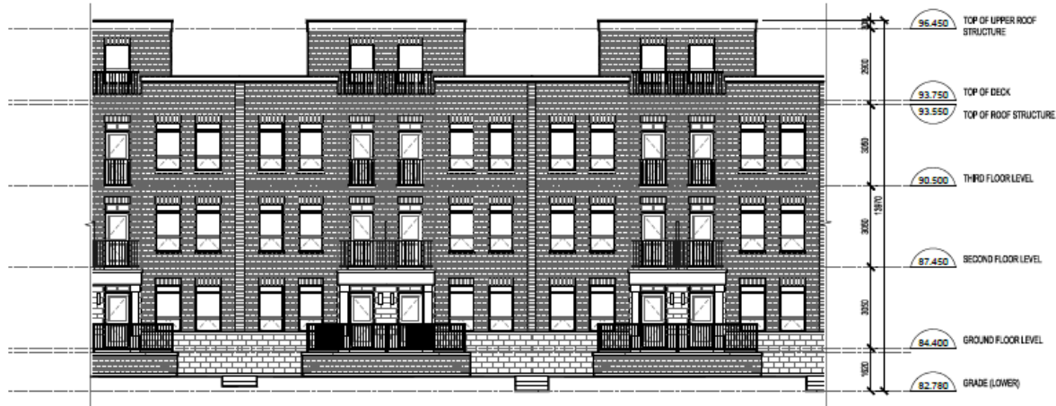
1 CONCEPTUAL WEST ELEVATION - OPTION 1 SK-4 SCALE: 1:150
