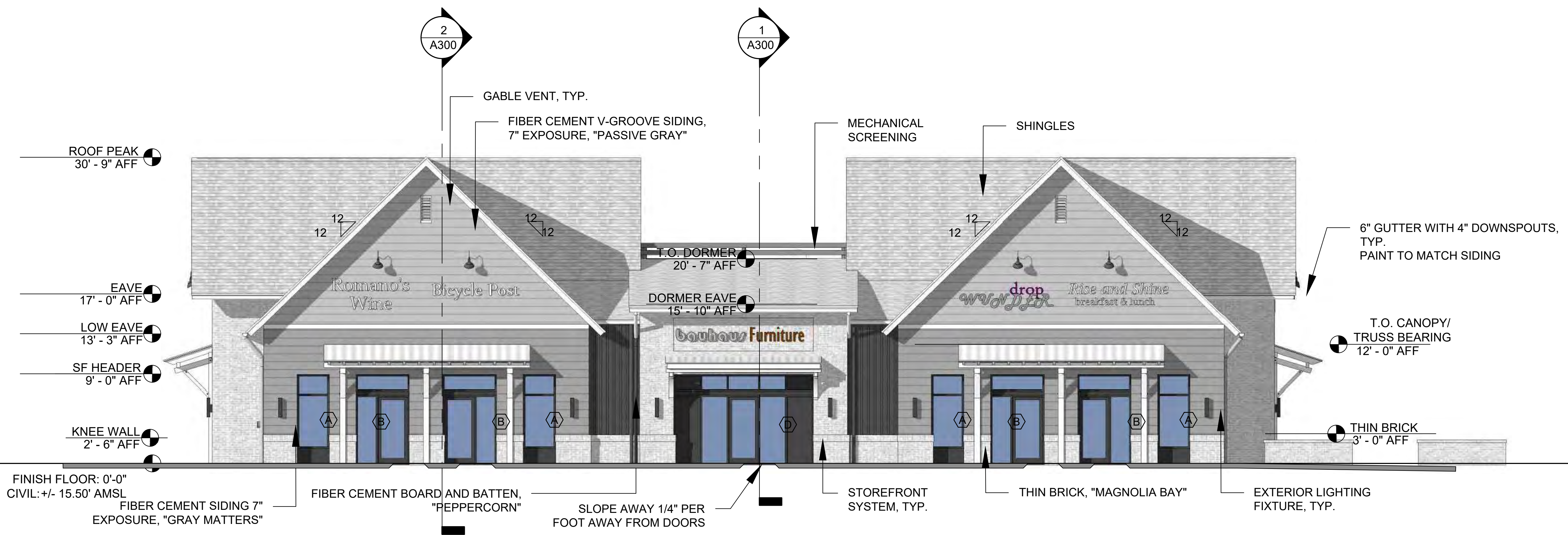
1 NORTH ELEVATION (REAR) SCALE: 3/16" = 1'-0"
