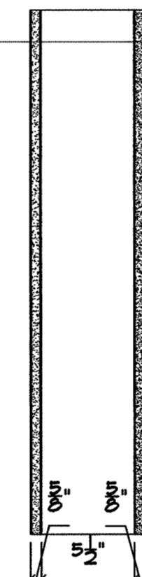
C 2X6 STUD W/ 1 LAYERS GYPSON BOARD A900 SCALE: 1/2"=1'
