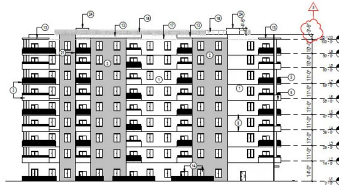
4 BUILDING A WEST ELEVATION SCALE: 3/8" = 1'-0"
