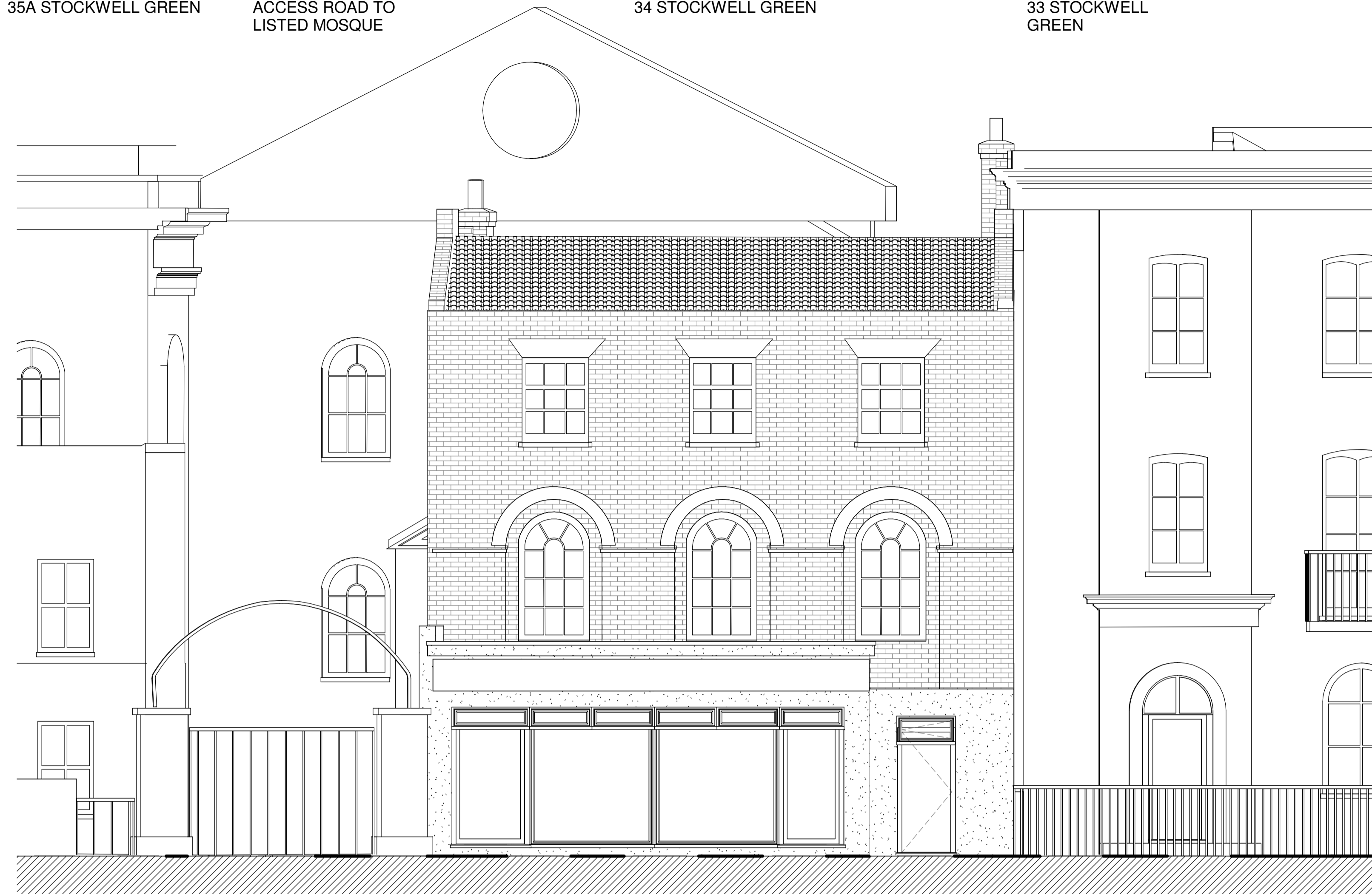
EXISTING FRONT ELEVATION 1:50
