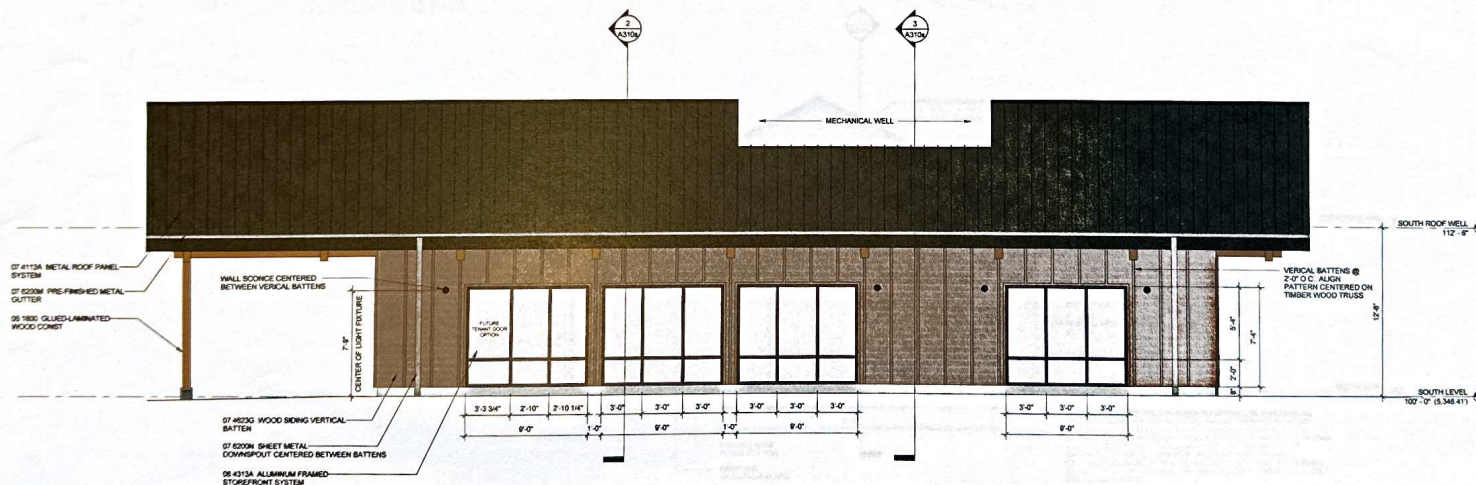
1 SOUTH ELEVATION - SOUTH A300s 1/4" = 1'-0"
