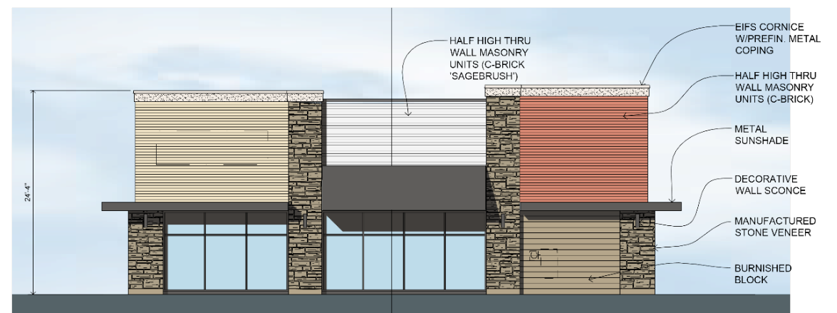
Bldg. A - East Elevation 1/8" = 1'-0"
