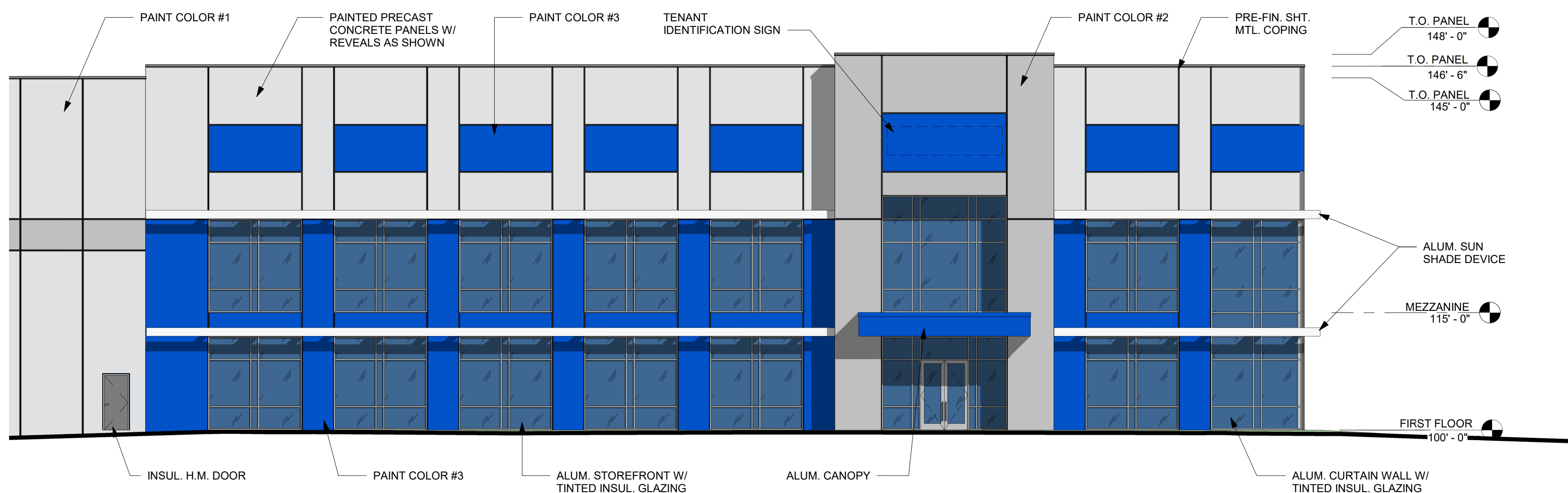
2 ENLARGED WEST ELEVATION 3/32" = 1'-0"
