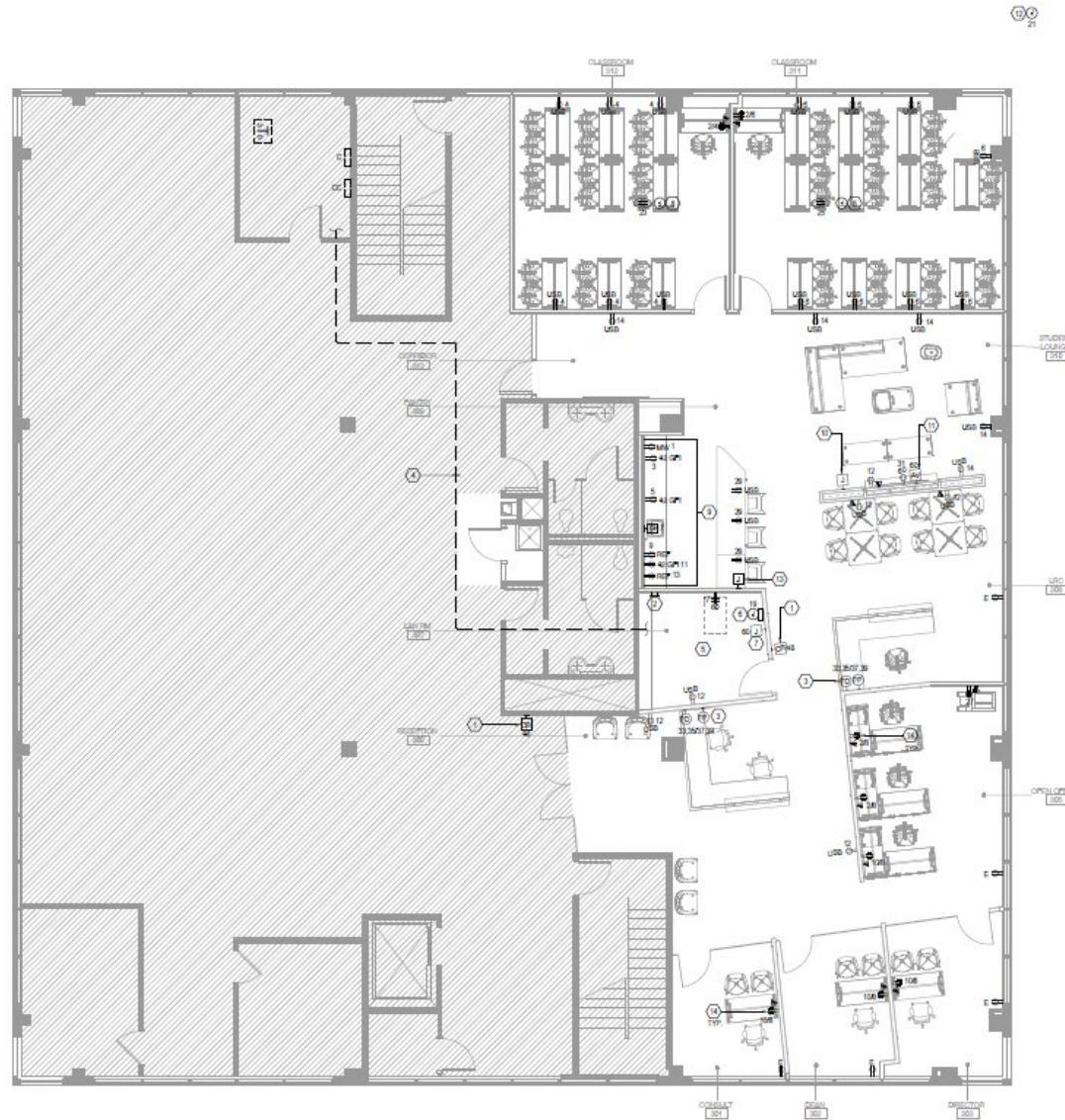
1 ELECTRICAL 3RD FLOOR POWER PLAN 3/16" = 1'-0"
