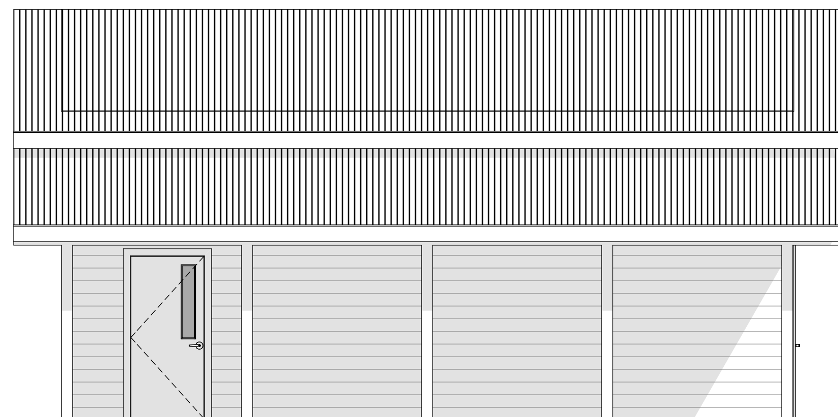
Storage/Utility Structure - Right Elevation | SCALE: 1/4" = 1'-0"
