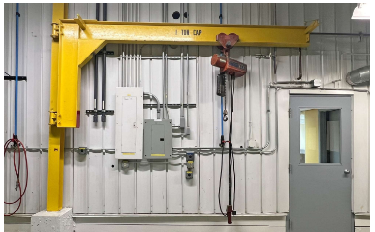
1-Ton Jib Crane With ±9'6" Under Arm & ±7'6" Under Hook
