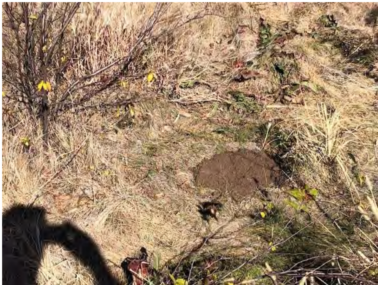
PLUGGED BORING SB-4
