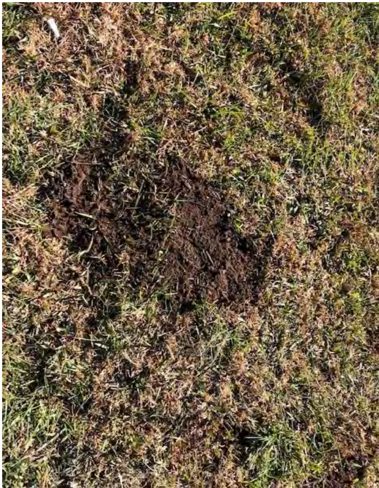
TYPICAL PLUGGED BORING IN GRASSY AREAS (SB-1, SB-2 AND SB-3)
