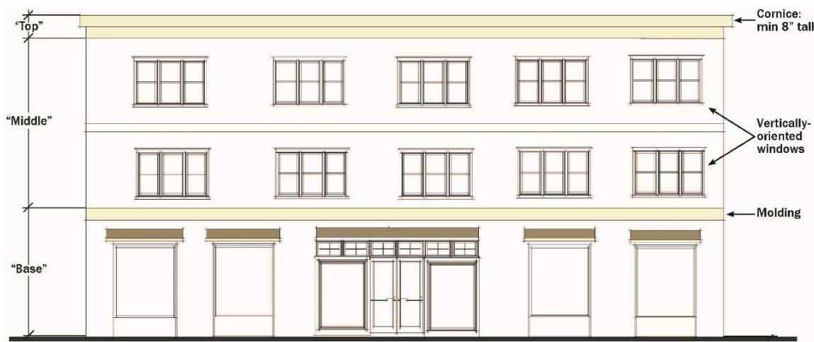
Ground Floor Windows
