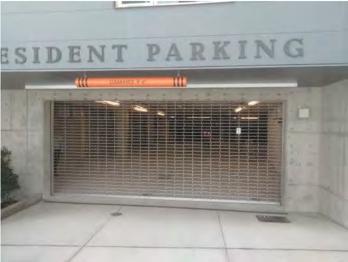
D-1 ROLL-UP SECURITY GRILLE MANUF: CORNELLCOOKSON TYPE: ROLL-UP SECURITY GRILLE: EXTREME MICROCOIL GRILLE-500K CYCLE OR EQUAL MATERIAL: STAINLESS STEEL; CUSTOM GRILLE DESIGN
