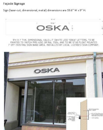
Figure 2: Sample of Section Drawing Showing Proposed Signage and Method of Installation
