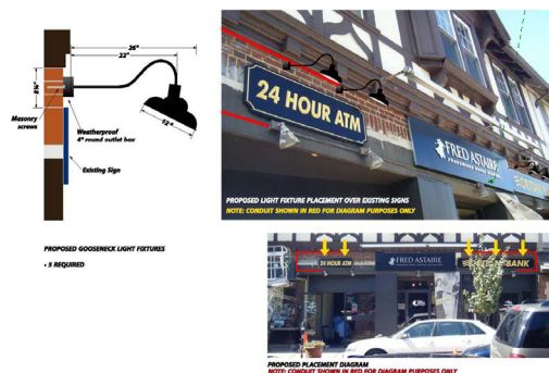
Figure 3: Sample of Lighting Details
