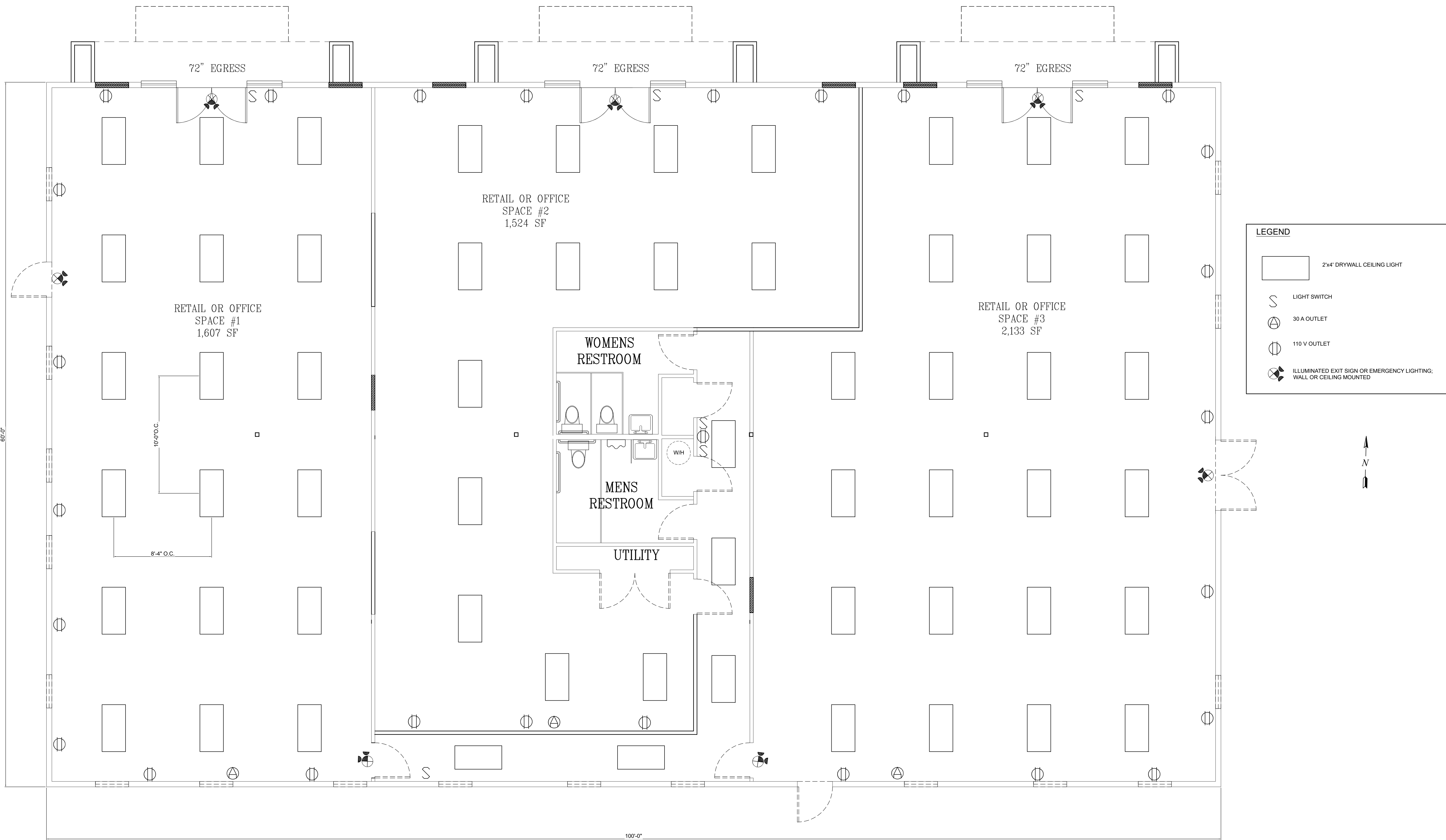
1 SAFETY MINIMUM LIGHTING PLAN BUILDING 14 SCALE: 1/4" = 1' - 0"
