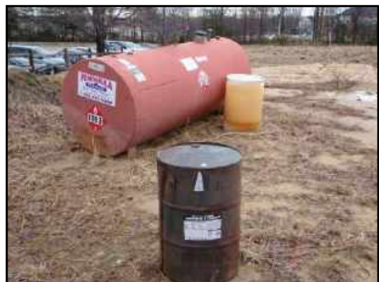
View of aboveground storage tank (1,000 gallons?) and two 55-gallon drums on northern side of site. The steel tank in the foreground was sealed and appears to be empty, and is labeled as containing anti-freeze. The plastic tank in the background was unmarked and had an open cap on the top; although mostly empty, there are contents that have a strong oil odor.
