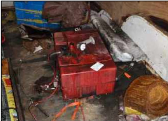
Small gas tank within small storage tank. There is a small amount of staining on the wooden floor of the storage trailer.
