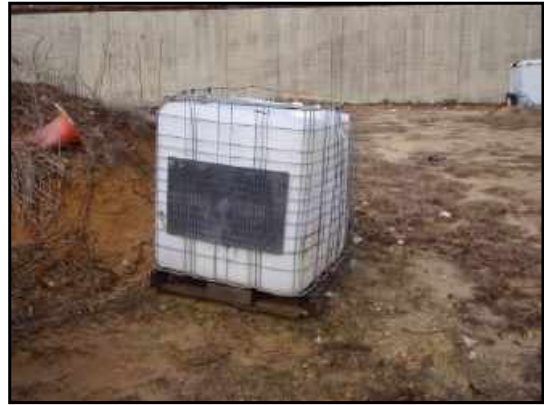
Plastic 275-gallon tote tank in the middle of the site. This tank is empty and unmarked. It is sealed. No staining beneath or spills were observed.
