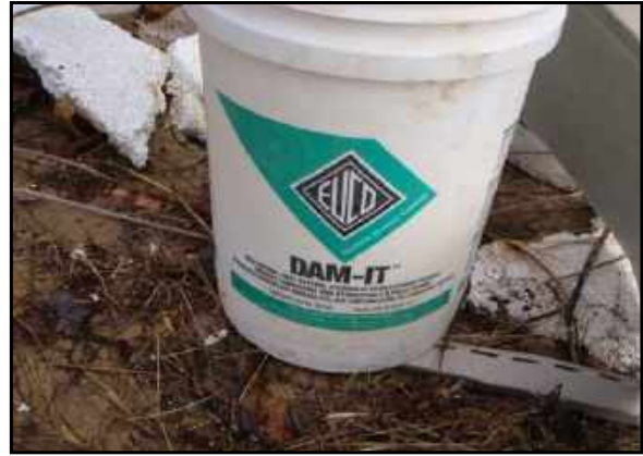
Hydraulic cement buckets.
