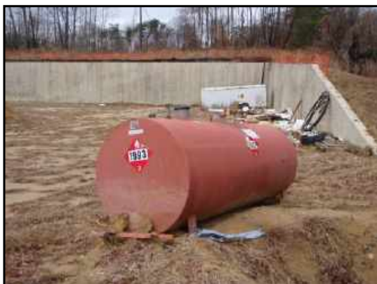
Aboveground storage tank, approximately 1,000-gallons in size (unmarked as to size) on site at central-northern portion of site. The tank appears to contain some petroleum product inside, with the cap off it may also be receiving rainfall. The tank appears to be in good condition and no spills, leaks or stained soils beneath area evident. The tank contains liquid with a strong petroleum odor.
