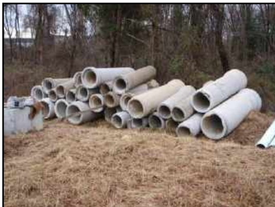
There are precast concrete pipes stored on the southern end of the subject property; these pipes do not appear to be new.
